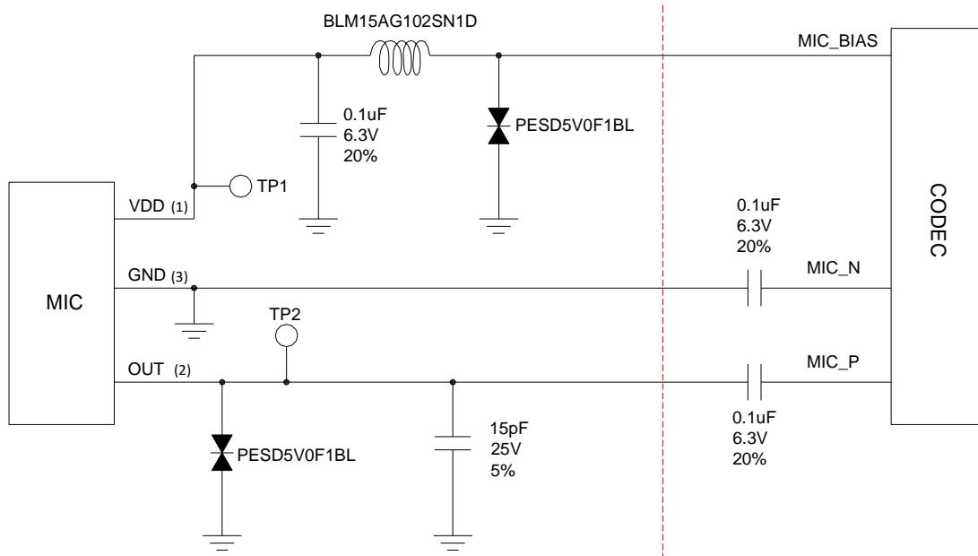
NOTE: It is recommended that the components on the left side of red line be placed close to MIC, and components on the right side of red line be placed close to codec.
