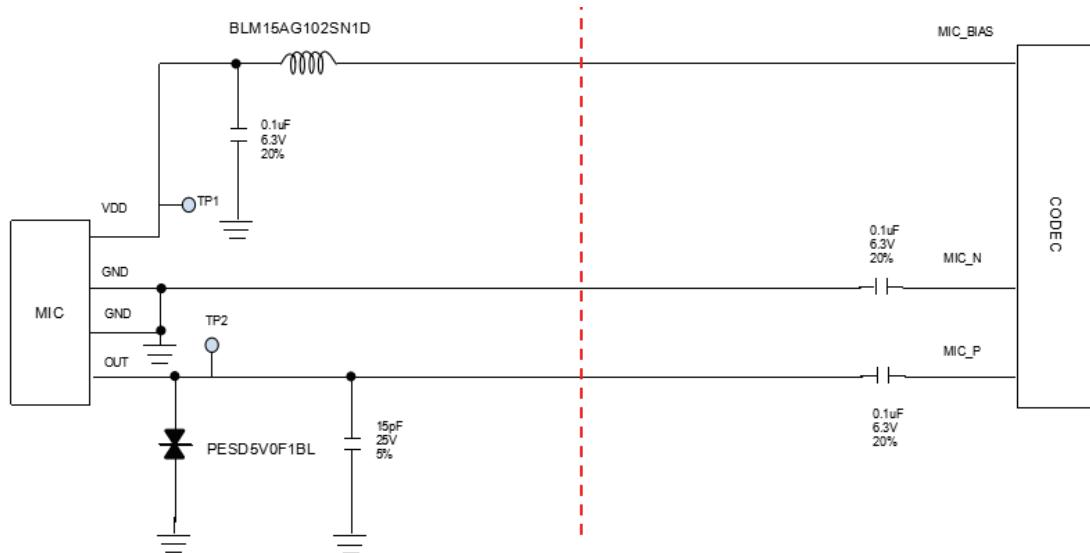
NOTE: It is recommended that the components on the left side of red line be placed close to MIC, and components on the right side of red line be placed close to codec.
