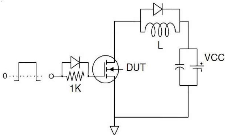
3) Switch Time Test Circuit:
