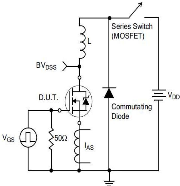
Figure17.Unclamped Inductive Switching Test Circuit
